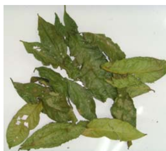
Tea leaves which were dried with pulsed microwave operating mode at 800 W magnetron power
